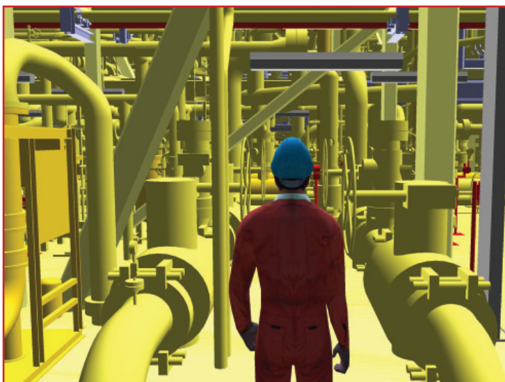
Figure 1. Surface facility in 3D with a human avatar, whose movements are subject to physical constraints, such as gravity and collision.
